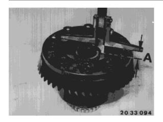
Install following parts in correct installed order to measure the preload:
