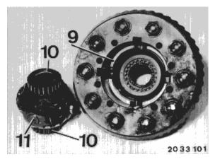
Install compression ring (9) and differential side gear (10) by twisting into the guide and/or spline of the inner disc.
