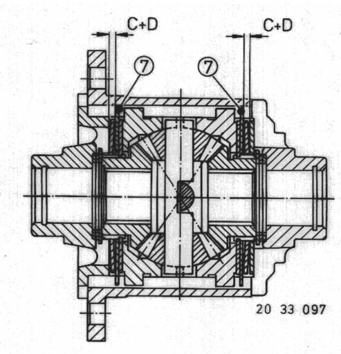
To ensure that the plate springs are not block-preloaded, installation clearance of 0.1 ... 0.4 mm is required.
